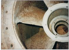
Severe erosion/ corrosion damage to pumps...
