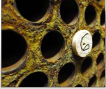
At the corporate headquarters of a major food manufacturer in Minnesota, three chillers had serious erosion and corrosion problems on the tube sheets and heads.
