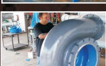
This pump, from a Los Angeles County power plant, had been suffering from extreme corrosion due to the pump's constant exposure to brine. Replacing the impeller alone would cost about \$50,000.
