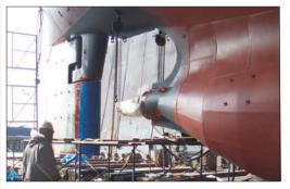
This large auto ferry had been experiencing severe cathodic corrosion damage in the The local ENECON keel cooler pockets. The ferry's engineers were unable to maintain recommended proper cathodic protection with standard as a solution. solid anode installations.
