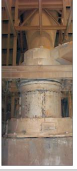
effective as well as longer hard face welding to protect the crusher components on their 66 inch Raymond Mill. They turned to ENECON's Coast Region for help. He suggested that they try CeramAlloy CBX to see if it would last longer than the chromium hard facing. The welding process is very expensive and time consuming and has a life expectancy of only about 10,000 tons of
