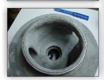
A municipal wastewater treatment plant in South Florida realized they had a problem with one of their pumps. These pumps work all day pumping "sewage, grease, sand, rocks, you name it," according to the plant engineers. Because of the harsh environment the impellers on these pumps take a severe beating.
