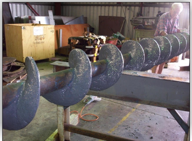
Screw conveyor protected with CBX
