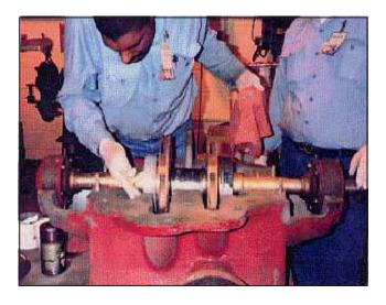
This Peerless deballasting pump from the floating dry-dock USS Sustain sat at the Shore Intermediate Maintenance Facility (SIMA) shop for over a year, awaiting an appropriate and acceptable solution. The estimated cost to cast an exact replacement of this unusual cast steel casing, built in 1944, was in excess of a quarter million dollars. A similar, more recent unit, which would have required extensive re-piping, would have cost over \$100,000.
