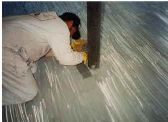
This commuter ferry operating in San Francisco Bay was experiencing an unusual problem. Its twin hull, catamaran design incorporates "tongue and groove" aluminum deck boards to span the area between the hulls. Salt water was coming up through the boards causing accelerated corrosion. In addition, the carpeting in the passenger compartment was constantly wet, resulting in complaints from the commuters and a potentially hazardous condition.
