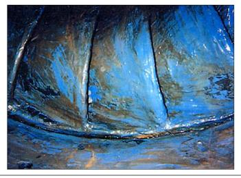
A hydroelectric plant in British Columbia, Canada, has found the use of our ENECON FLEXICLAD DuraTough to be the best method of repairing and protecting these Francis Turbine Runners from severe cavitation attack.
