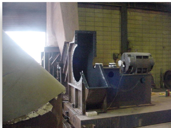
Two coats of CHEMCLADSC were applied to all interior surfaces and flanges.
