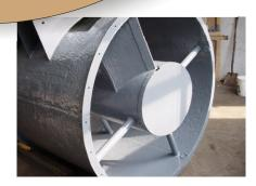
Scott Tresser, the local ENECON Distributor in Pittsburgh, was asked to salvage a 66" diameter x 60" long fan housing belonging to a local rendering plant. The fan draws air into a scrubber to reduce the odor that is a result of the processing.
