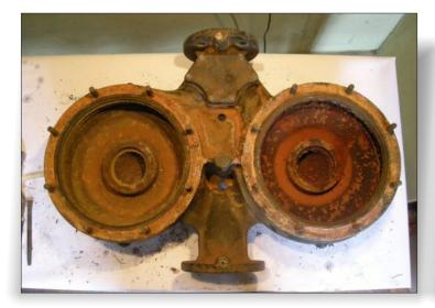
This hard water pump at a hospital in Chile was only averaging a few months in service before maintenance would have to be performed to repair deep erosion / corrosion damage.
