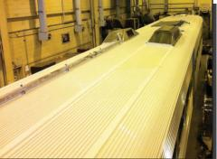
Solution: The surface was prepared by high pressure washing and the seams were sealed with a silicone caulk. ENESEAL CR was applied as a surface primer followed by two coats of ENESEAL HR.
