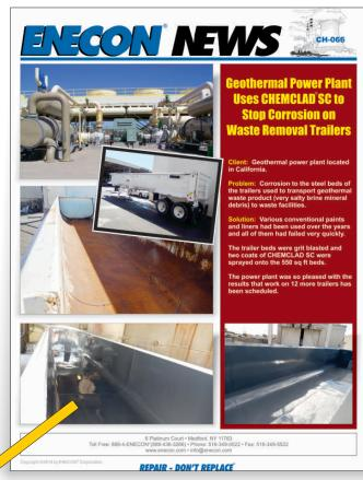
After one year in service transporting extremely corrosive brine mineral debris, the trailer beds are showing no signs of corrosion. Other products previously tried only lasted a few months.
