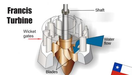
These wicket gates for a Francis turbine, used in the hydroelectric industry, direct high flowing water so it hits the blades of the turbine at the most efficient angle. They suffer from constant erosion / corrosion when they are not protected properly. Most companies would toss worn wicket gates into their 'bone yards' and buy very expensive new gates for their turbines. ENECON Chile was contacted to prescribe a more cost effective and fast solution.
